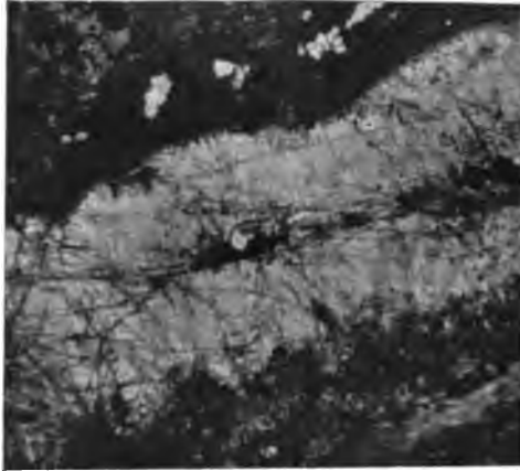
A. HANCOCK LODGE. PHOTOMICROGRAPH. THIS SECTION SHOWS NATIVE COPPER IN RATHER LARGE PARTICLES ALONG THE MIDDLE OF A VEIN OF PREHNITE. COPPER OCCURS ALSO IN SMALL PARTICLES IN THE ROCK ON EITHER SIDE OF THE VEIN.
